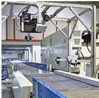
The XS100 DualScale offers high-speed, high-throughput weighing in the most demanding of applications. Rugged design and advanced filter technology ensure stable, accurate results even when conditions are tough.
